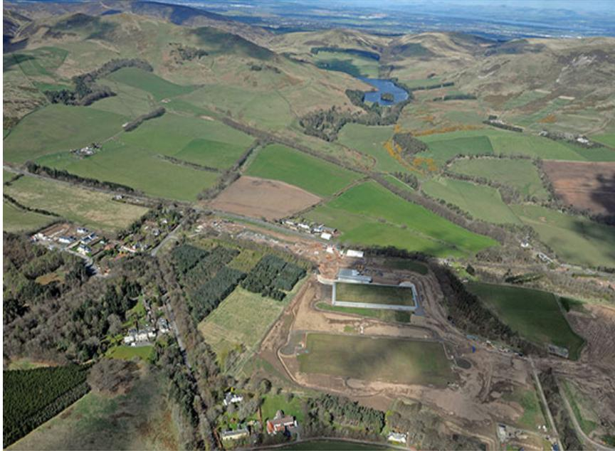
Glencourse supplies fresh drinking water to around 450,000 customers across Edinburgh. Water pressure and flow within the assets is used to drive turbines to generate electricity. This integration into existing civil infrastructure provides a benefit in reduced construction cost compared to a standalone project.
