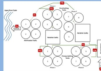
**Fig 1.** Sampling scheme in the tertiary STP for 8 sampling points: P1, influent; P2, pre-treatment effluent; P3a and P3b, primary effluent phases 1 and 2, respectively; P4a and P4b, secondary effluent phases 1 and 2; P5, secondary effluent, mixed liquor; P6, final effluent
