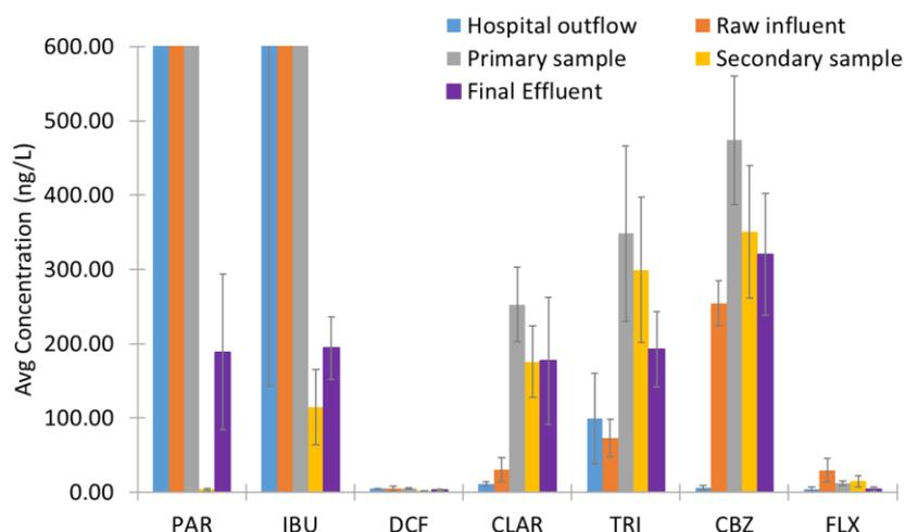
**Figure 1: Average (avg) concentrations of pharmaceuticals in ng/L detected at separate stages of the wastewater treatment process. Error bars indicate standard deviation (n=7). PAR = paracetamol, IBU = ibuprofen, DCF = diclofenac, CLAR = clarithromycin, TRI = trimethoprim, CBZ = carbamazepine, FLX = fluoxetine.**
