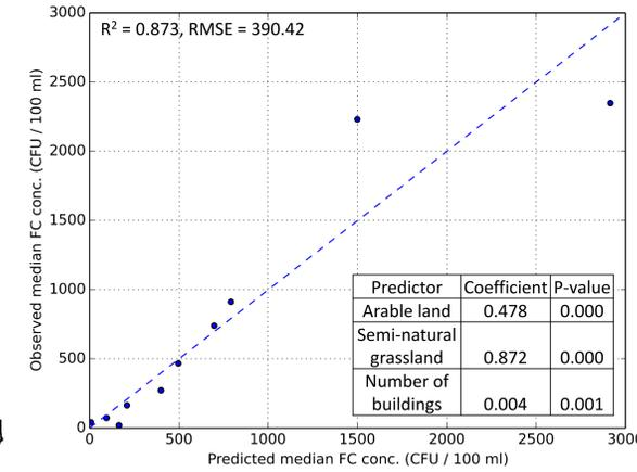
Fig. 4: Predicted vs. observed median FC conc.s obtained with Poisson regression model. Inset are predictor coefficients and performance metrics.
