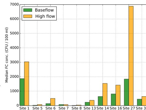
Fig. 6: Median FC conc.s under baseflow and high flow conditions.
