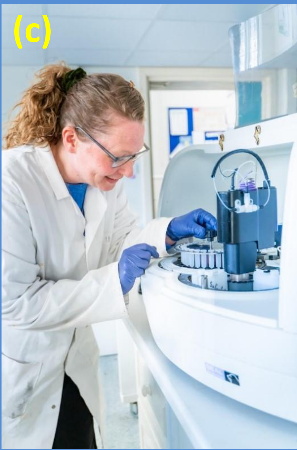
(a) Grab sample taken from river; (b) water sample about to be filtered; (c) AQ2 discrete analyser.
