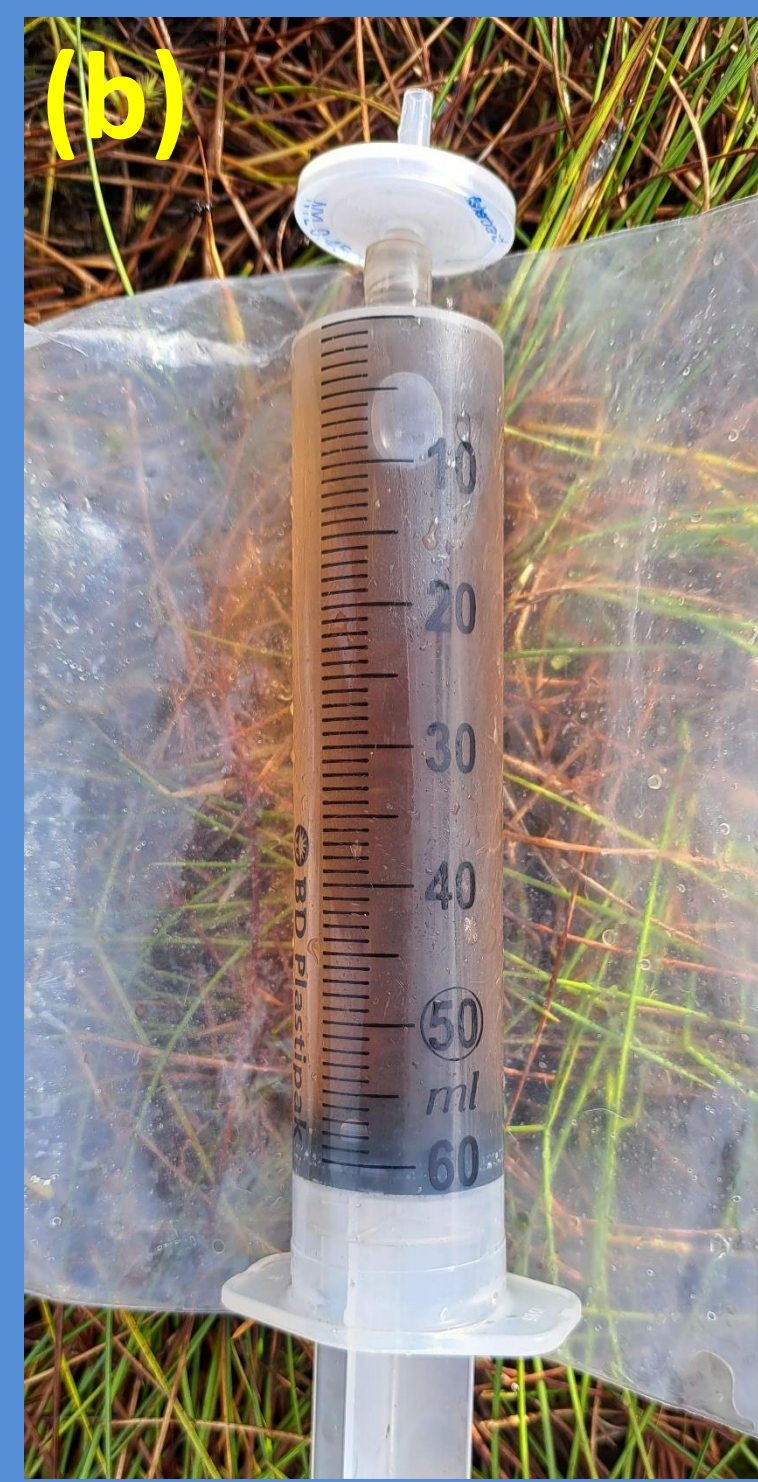
(a) Grab sample taken from river; (b) water sample about to be filtered; (c) AQ2 discrete analyser.
