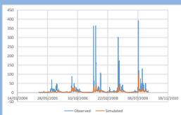
Figure: Observed and Simulated stream flow time series for the gauging station– Thimmanahalli, Upper Cauvery
