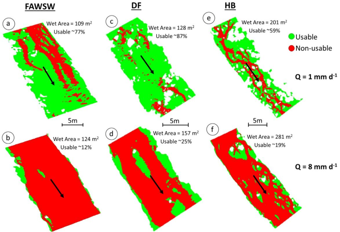
Fig. 5. Usable and non-usable habitat under two contrasting flow conditions: one low (1 mm d<sup>-1</sup>) and one high (8 mm d<sup>-1</sup>) for FAWS, DF, and HB.
