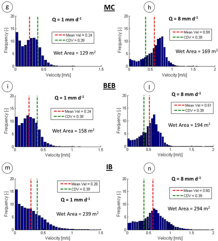
Fig. A.2. Velocity distribution, wetted area and mean water velocity under two contrasting flow conditions: one low ( $1 \text{ mm d}^{-1}$ ) and one high ( $8 \text{ mm d}^{-1}$ ) for MC, BEB, and IB.
