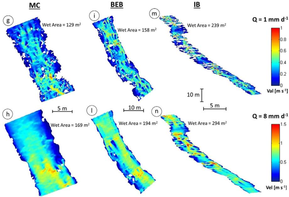
Fig. A.1. Simulated spatial distribution of water velocity under two contrasting flow conditions: one low ( $1 \text{ mm d}^{-1}$ ) and one high ( $8 \text{ mm d}^{-1}$ ) for MC, BEB, and IB sites.
