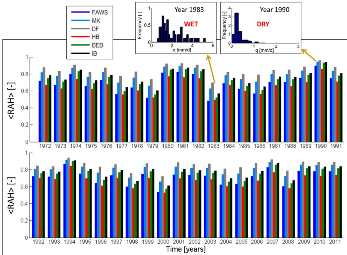
Fig. 7. <RAH> from 1972 to 2011 for all sites; and examples of two contrasting flow regimes providing greater (DRY) and lower (WET) <RAH>.
