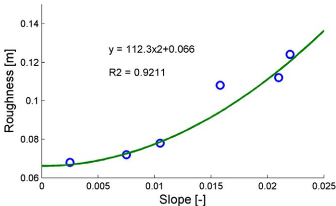
Fig. 8. Estimated slope vs. estimated roughness and corresponding fitting curve.
