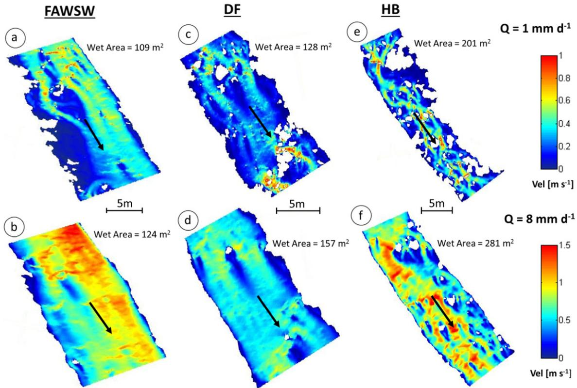
Fig. 3. Simulated spatial distribution of water velocity under two contrasting flow conditions: one low ( $1 \text{ mm d}^{-1}$ ) and one high ( $8 \text{ mm d}^{-1}$ ) for FAWS, DF, and HB sites.
