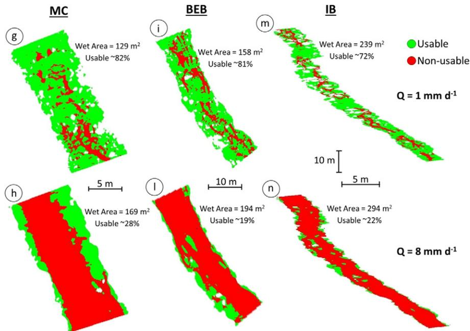
Fig. A.3. Usable and non-usable habitat under two contrasting flow conditions: one low ( $1 \text{ mm d}^{-1}$ ) and one high ( $8 \text{ mm d}^{-1}$ ) for MC, BEB, and IB.
