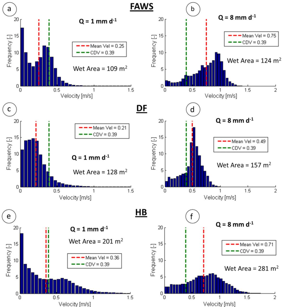
Fig. 4. Velocity distribution, wetted area and mean water velocity under two contrasting flow conditions: one low ( $1 \text{ mm d}^{-1}$ ) and one high ( $8 \text{ mm d}^{-1}$ ) for FAWS, DF, and HB.
