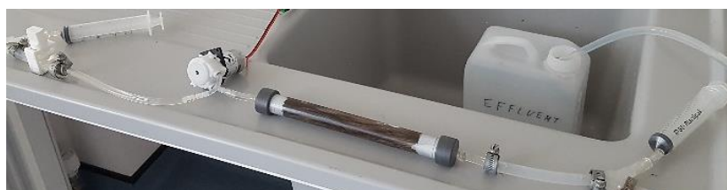
Experimental rig design with nanomaterial filter cartridge from PolyCatUK Ltd.
