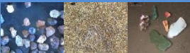
Figure 2 Non-polymer micropellet (left), MP fibres (middle), and non-polymer and MP fragments (right) found in River Kelvin sediment sampled December 2015 and February 2016. Non-polymer pellets and fragments can be misidentified as primary and secondary MP, respectively, by visual inspection alone, while fibres and smaller fragments (secondary MP) need DS & SEM to be quantified properly.
