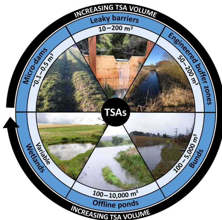
FIGURE 1 Types of small-scale headwater temporary storage areas (TSAs).
