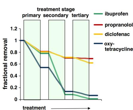
Figure 1. Depiction of influent concentrations (%) removed during separate stages of the WWT and discharged in effluent (Gardner et al., 2013)
