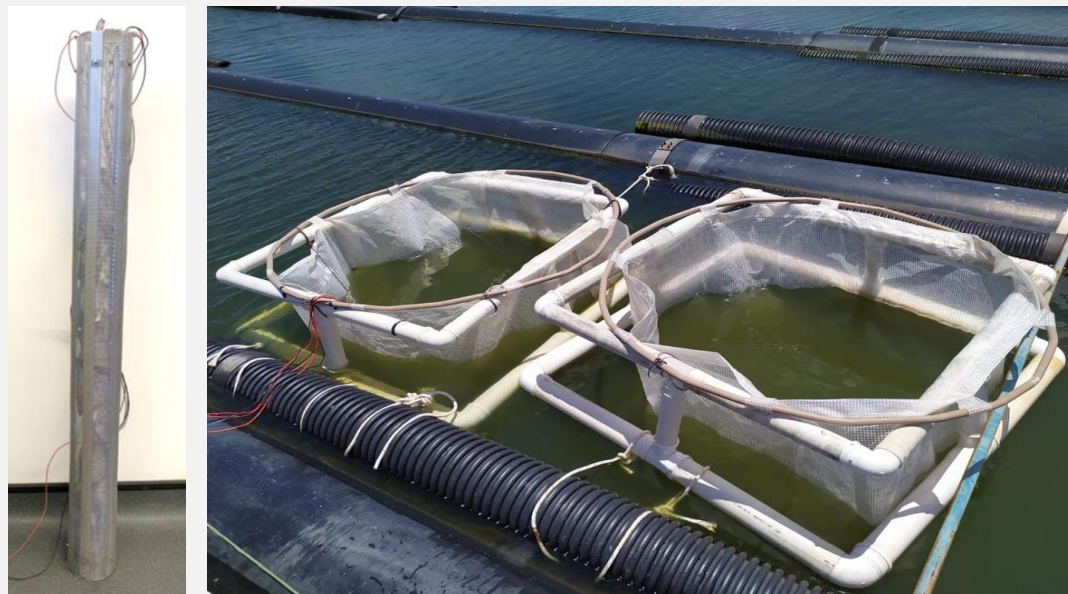
Fig. 2 – (Left) Initial treatment unit prototype proposed for the photocatalytic treatment unit for the degradation of pesticides at source. (Right) Mesocosms structure inside of the Gavião reservoir in Brazil containing photocatalytic treatment units in order to improve water quality and remove cyanotoxins.
