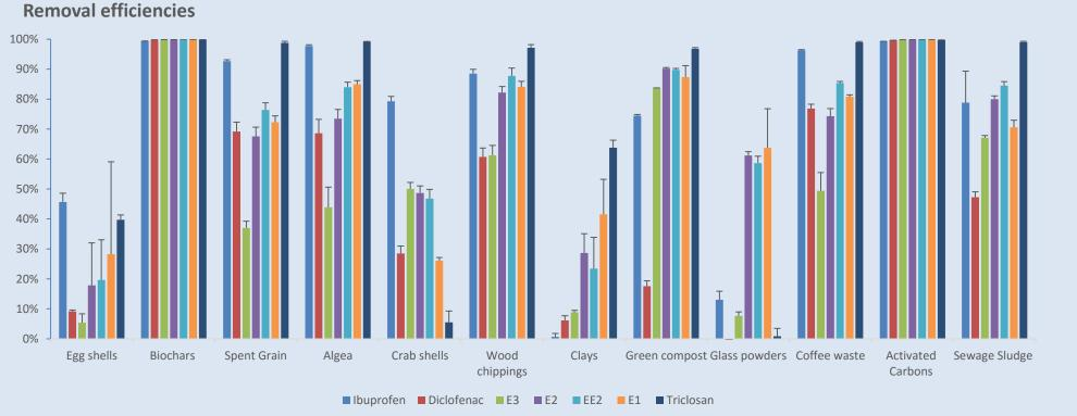
Figure3. Mean removal efficiencies of negatively ionised target compounds by 12 tested biosorbents (vertical error bars stand for 1 standard deviation)
