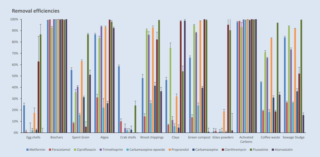
This project aims to utilize a variety of recycled industrial, domestic and agricultural by-products as low cost biosorbents for the removal of EDCs and PPCPs from wastewater. These will be used to develop dynamic, rechargeable column systems for wastewater effluents in pilot studies with Scottish Water and the Chinese Academy of Sciences. It is anticipated that the polishing treatment system will be applicable in rural or semi-rural (low flow) WWTPs in a fast and inexpensive way.
